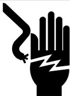
**Disconnect power from unit and wait at least five minutes to allow capacitors to discharge before attempting to adjust motor speed tap settings. Failure to wait may cause personal injury or death.**
